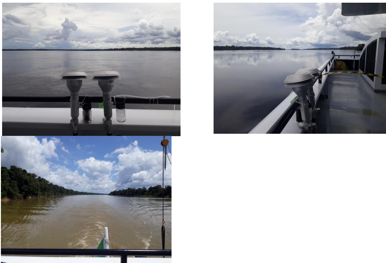
Figure 5.101 - Photos of the aerosol and gas inlets installed on the boat at the University of the State of Amazonas (UEA).
